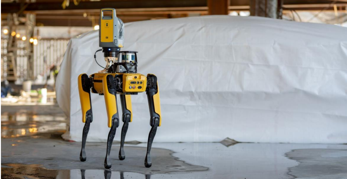
Figure 17: SPOT robot from Boston Dynamics with mounted laser scanner (BostonDynamics, n.d.)
