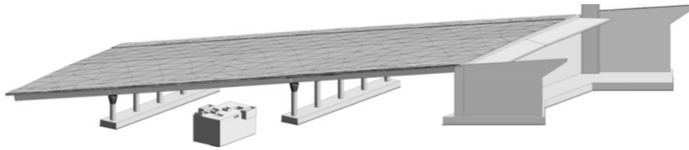
Figure 14: Geothermal modules under the Cardenal Herrera Oria bridge
